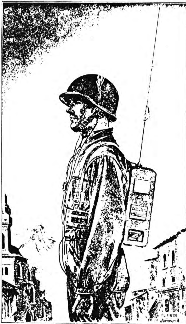
Figure 2. German radio set Feldfu. b, ready for operation.
