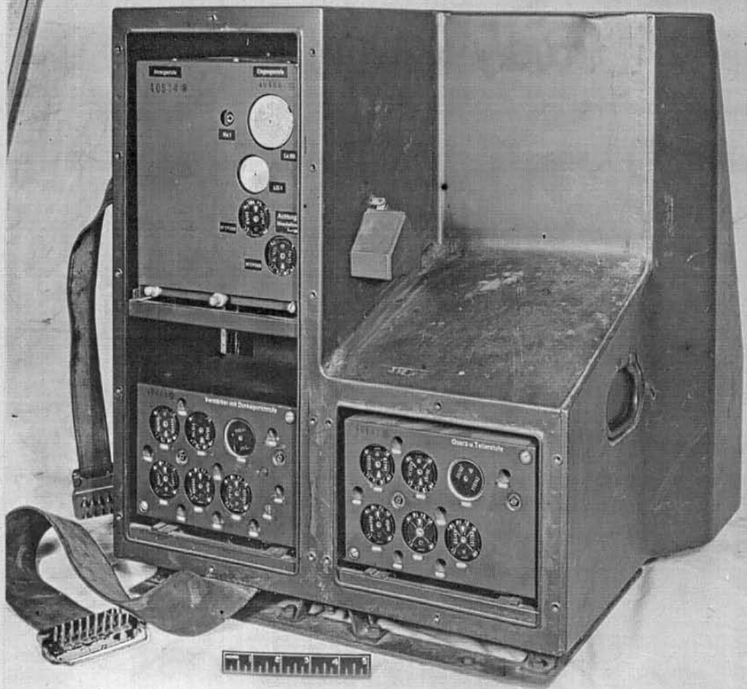
RANGE-MEASURING UNIT EAG 62. BACK VIEW WITH COVER OFF.
