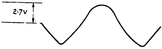
(b) OUTPUT OF VALVE 402 AT TERMINAL b3.
