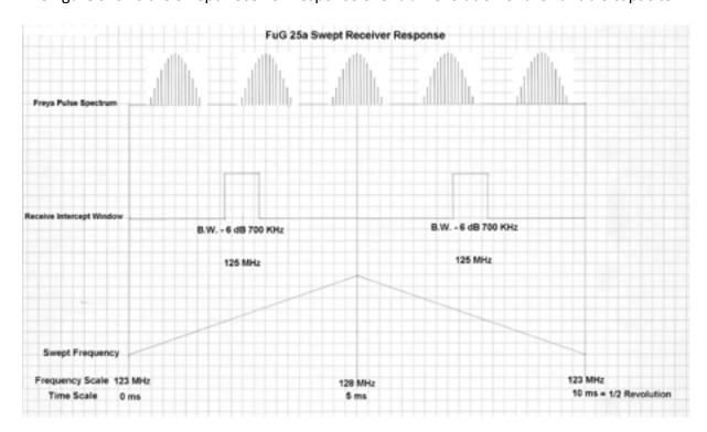
The figure shows that during one revolution of the variable differential capacitor the receive frequency sweps 4 times over the frequency band within a time interval of 20 milliseconds. As for instance the Freya pulses radiated with a prf of 500 Hz equal a time interval of 2 ms are intercepted by the FuG 25a receiver, if parts of their frequency spectrum are in step with the receivers interception windows.
