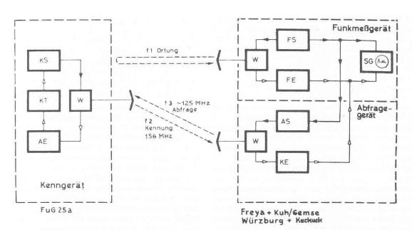
While its primary use was for identification purposes with the Freya radar it could also be used together with radars operating on other frequency bands, however for that purpose the 125 MHz interrogation transmitter « KUH » was necessary. Later in WWII the FuG 25a was also employed as bombing – release controller as well as for ground to air communication (Order Transmitter Apparatus).
