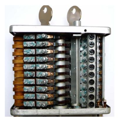
There are ten cams connected in parallel, each covering an adjacent 30°. Normally the contacts operated by these cams close in rotation, with slight overlap, so that the set would be on for % of a revolution and off for %. The period of rotation is about one and one - half seconds. The coding is obtained by lifting the contacts off any o the 10 cams, using a key for this purpose.
