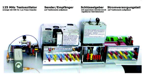
This measure allowed to open the circuits temporarly for measurements, stop specific functions as well as get better access to certain components. On the test adapter the code keyer could be operated with variable speed for specific experiments.
