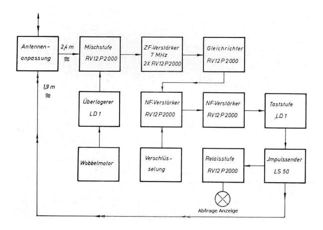
The receiver is an eight tube superheterodyne type that swept (Wobbeln in German) over the band 123 – 128 MHz at 200 Hz by a motor turning at 3000 rpm a variable differential capacitor in the local oscillator (Ueberlagerer) circuit.
