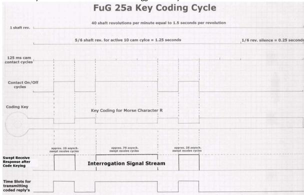
The FuG 25a transmitter is triggred by a combination of swept receive cycles and the key code. Caused by the 500 Hz prf of the Freya radars the FuG 25a transmitter migth be triggered up to 25 times during one cam contact cycle of 125 milliseconds.
